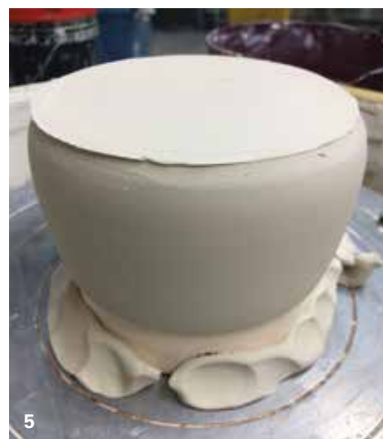
Using the moist clay helps protect the lip of the ramekins as you trim them.
